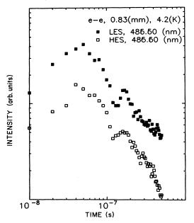
FIG. 4. Logarithmic plots of temporal responses of the bound-to-bound and free-to-bound transitions at the A-exciton resonance  $\lambda_{exc}$  = 485.6 nm for the 0.8-mm CdS sample at T = 4.2 K.
