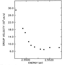
FIG. 3. Experimentally observed polariton group velocities vs excitation photon energies at 4.2 K for the 2.6-mm CdS sample.
