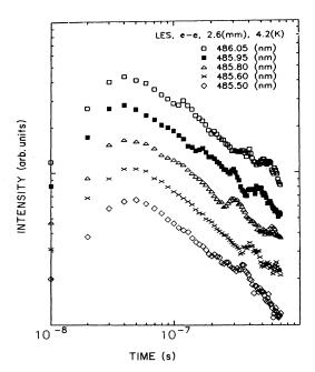
FIG. 1. Logarithmic plots of temporal responses of the bound-to-bound transition for various excitation photon wavelengths in the vicinity of the *A*-exciton region at 4.2 K for a 2.6-mm CdS sample.
