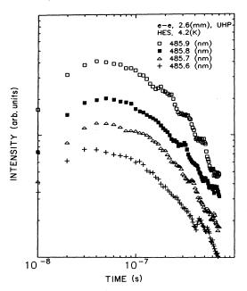
FIG. 2. Logarithmic plots of temporal responses of the freeto-bound transition for various excitation photon wavelengths in the vicinity of the A-exciton region at 4.2 K for a 2.6-mm CdS sample.
